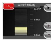
The electrical current applied by the electrodes is displayed both as numerical values and on a logarithmical scaled graph.
