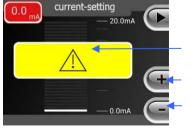
Caution! Current interrupted; check cable and sockets
